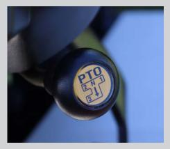
Convenience of a 3 speed PTO at 540, 750 and 1000 rpm. A speed for every job
