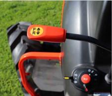
Well placed forward/reverse shuttle lever for ease of operation
