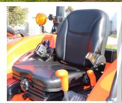
Adjustable mechanical suspension seat makes operation more comfortable
