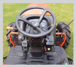
A flat operator station, with a tilt steering column and ergonoically placed controls
