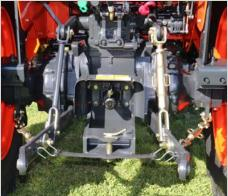
A rear lift capacity of 1334 kg and a lever to operate the linkage from the rear of the tractor. Two sets of rear hydraulic remotes come standard
